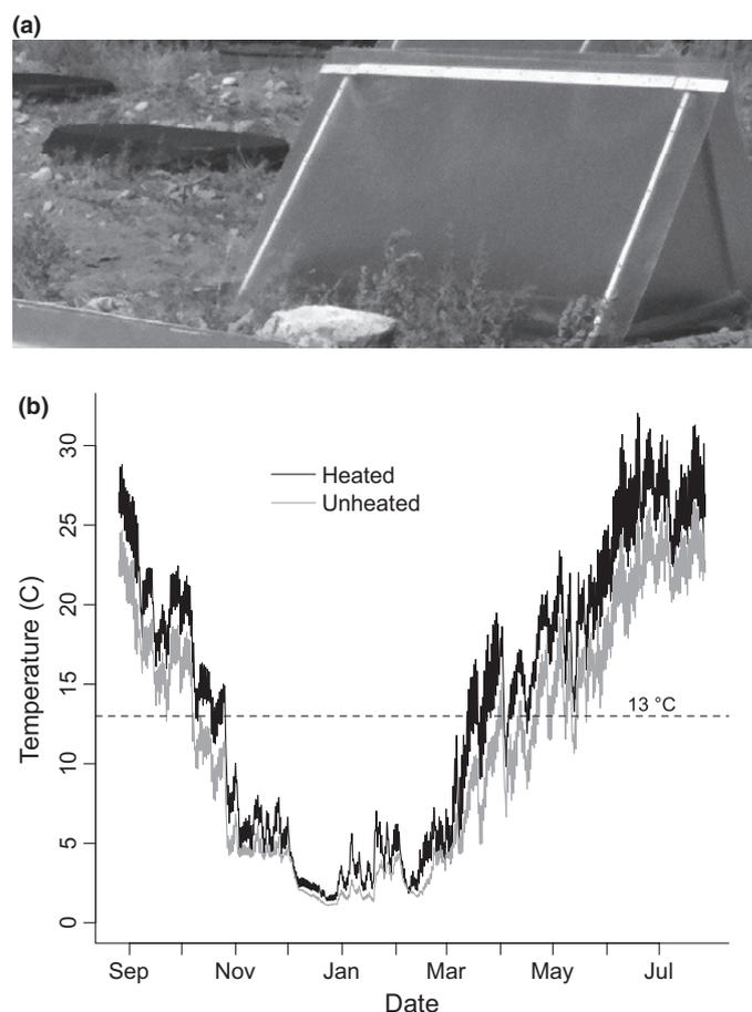
**Figure 1** Photo of (a) and seasonal water temperature profile in (b) outdoor mesocosms (379 L) either unmanipulated or heated using greenhouse lids. The dashed line at 13 °C indicates the threshold temperature below which infected snails stop releasing parasites (Paull & Johnson 2011).
